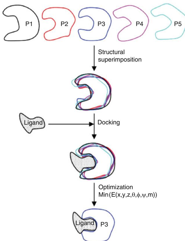
**Fig. 5** A cartoon illustration of ensemble docking, where five individual protein structures are superimposed to create a single scoring parameter for the docked ligand. Ensemble docking minimizes the computational effort since a single docking occurs to select the best conformer instead of five separate molecular docking simulations. (Reprinted with permission from [118], copyright 2007 by John Wiley and Sons)
