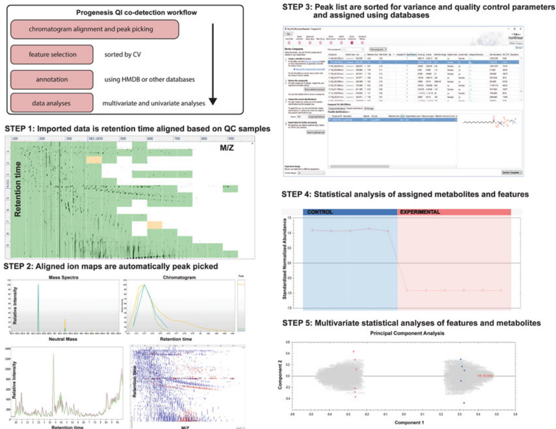
Fig. 9 LC-MS processing protocol. The small molecule discovery workflow using the Progenesis QI software is diagrammed. ( top left ) Summary of the major steps in the LC-MS processing protocol, which also describes each figure block in order starting from middle-left to bottom-right . Images are screenshots from the Progenesis QI software
