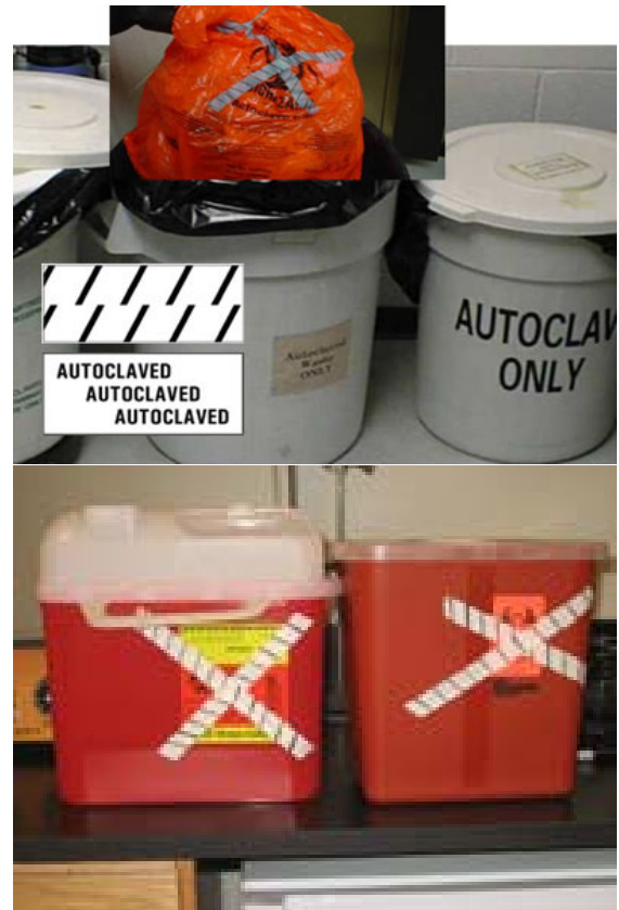
Figure 1 Autoclave tape utilizes a chemical reaction to indicate a temperature of greater than 121°C was achieved. This color change is usually displayed with hash marks or words that appear on the tape when proper temperature is reached.
